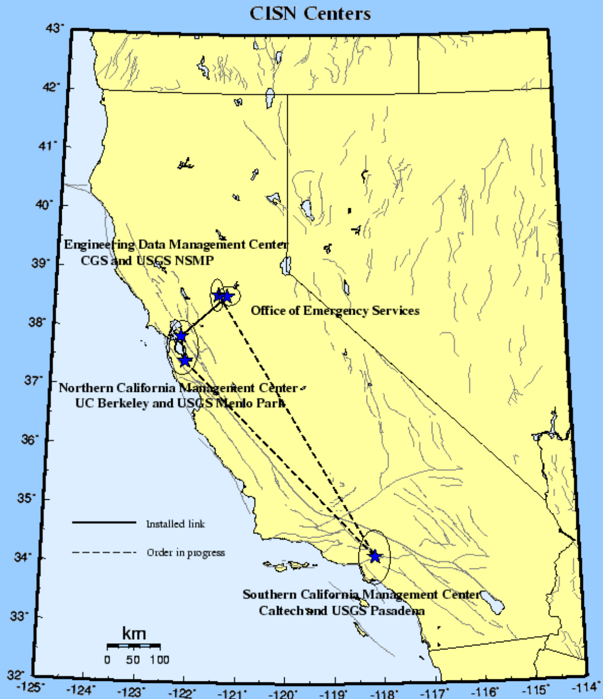
"Map showing the geographical distribution of the CISN partners and centers. The communications "ring" is shown schematically with installed links (solid lines) and ordered links (dotted lines)". ( CISN 2007-2008 Activities )
